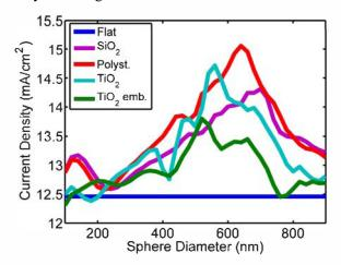
Fig. 3. Current density as a function of the sphere diameter for each considered case.
