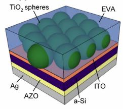
Fig. 1. Schematic of the solar cell with  ${\rm TiO_2}$  spheres embedded in EVA.
